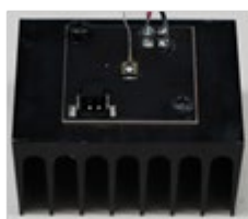
Picture 9: Fins Point Downward (Airflow is Blocked).
